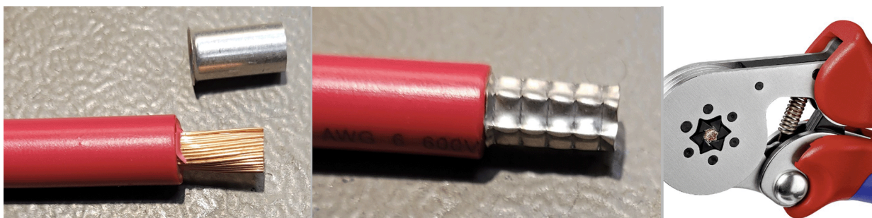
Hexagonally crimped bootlace ferrule
